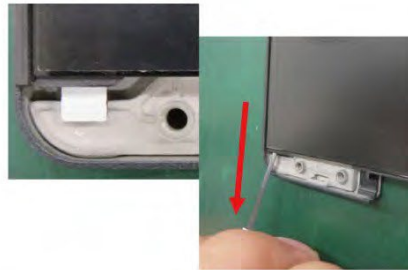
⑥D TAPE TP SIDE L Pull toward the arrow pointing
