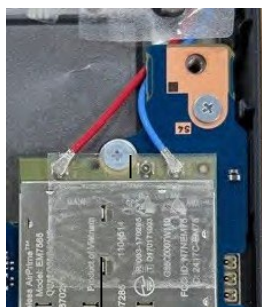
Figure 4-9 Removing the 5G/LTE MODULE
