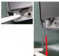
④D TAPE TP LS L Pull toward the arrow pointing
