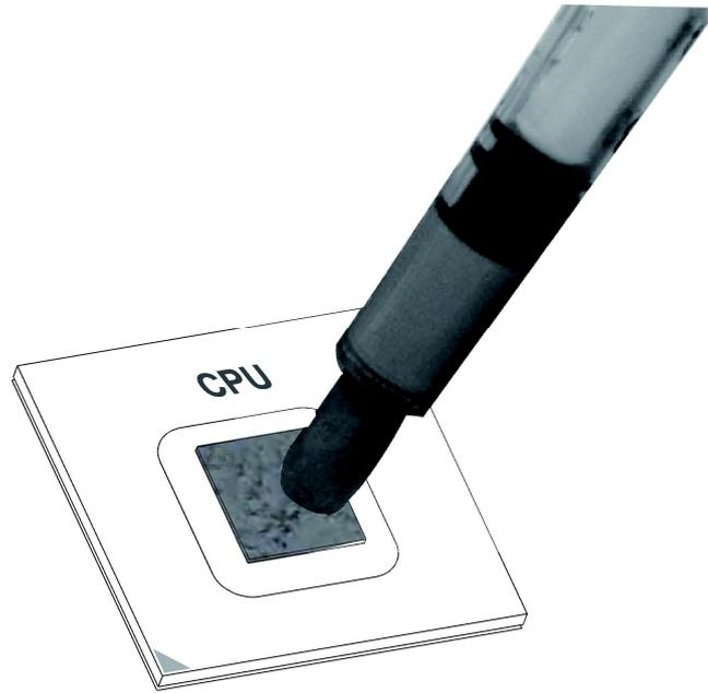
Figure 4-20 Applying silicon grease
