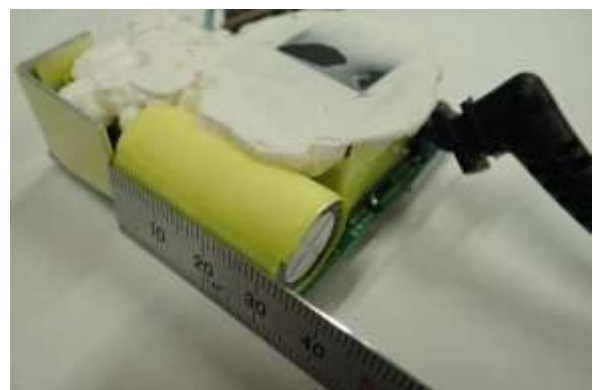
AC adapter capacitor
