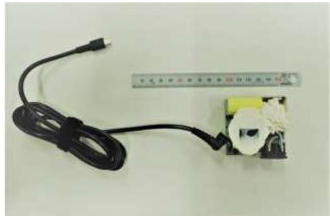
*AC Adapter with casing removed*
