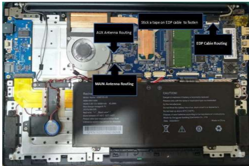
Figure 4-18 Removing the LCD Module assembly
