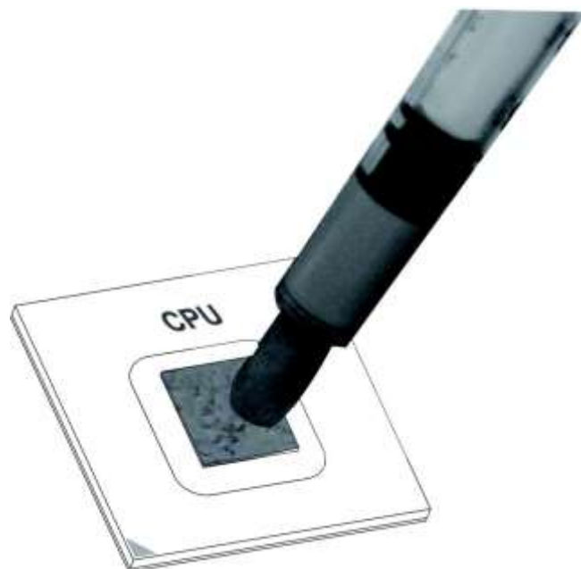
Figure 4-20 Applying silicon grease
