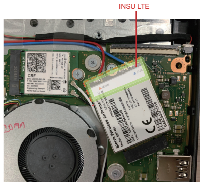
Figure 4-20 Installing the 3G module
