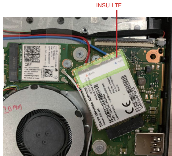
Figure 4-20 Installing the 3G module
