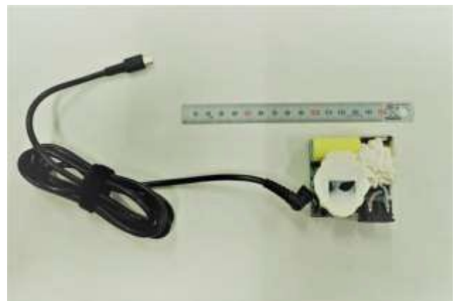
AC Adapter with casing removed
