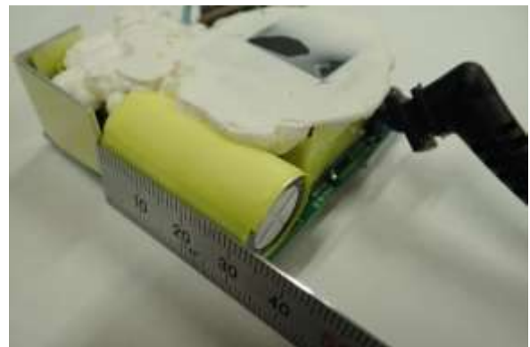
AC adapter capacitor
