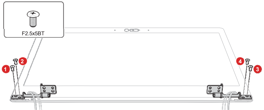
Figure 4-46 Installing the LCD unit (3)
