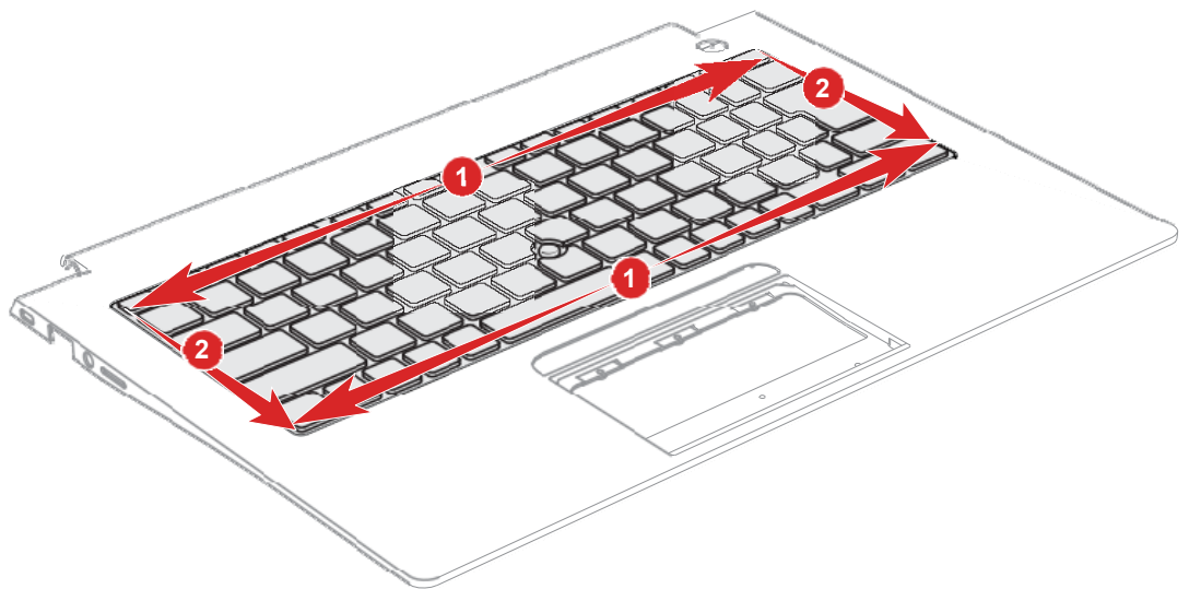
Figure 4-48 Installing the keyboard (7)
