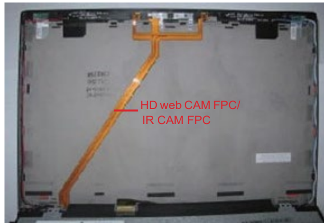
Figure 4-59 Removing the camera module (3)
