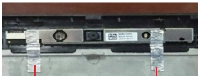
Figure 4-59 Removing the camera module (1)
