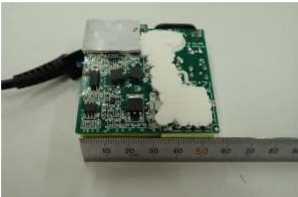
*AC Adapter printed circuit board*
