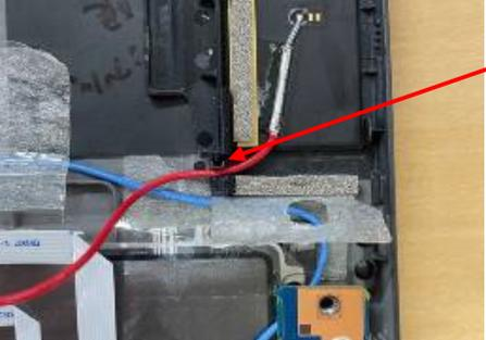
Insert the MAIN cable (red) to the rib.
