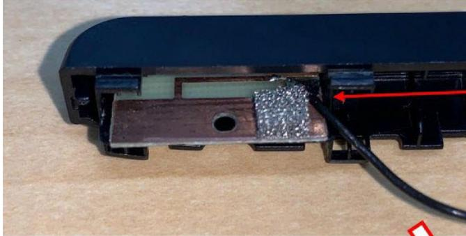
Stick the W-LAN AUX ANTENNA to the end of the CORNER CAP L.
