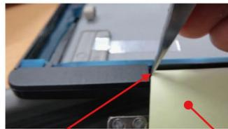
Insert the tweezers between the HINGE CAP and HINGE CASE.
