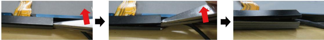
Insert the tweezers and lift it up to release the latches.
