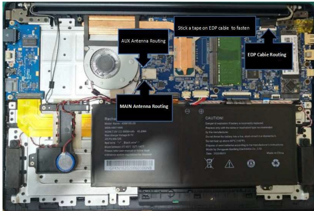
Figure 4-18 Removing the LCD Module assembly
