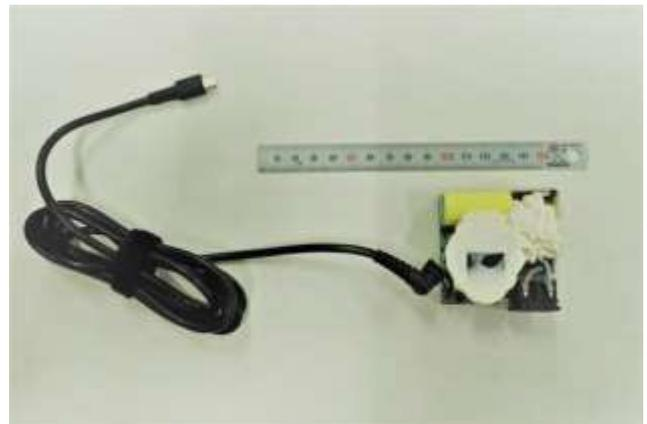
*AC Adapter with casing removed*
