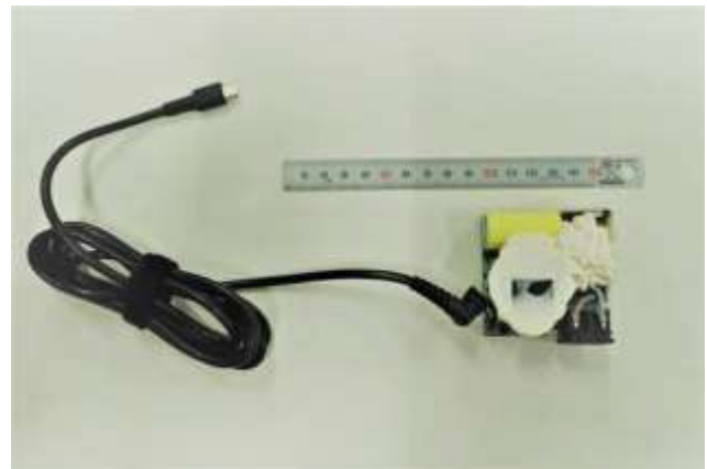
AC Adapter with casing removed
