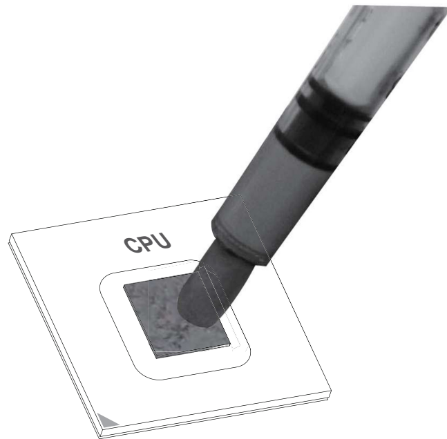
Figure 4-14 Applying silicon grease
